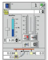
coating efficiency and performance. With Smart Flow, optimum "velocity" of the spray pattern for the particular part being coated is set first; then, the powder output level is set to achieve the desired film thickness on the part.
