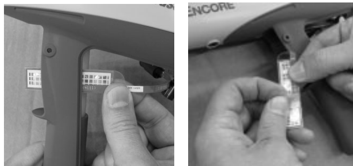
Figure 6-9 Installing the Trigger Switch – Steps 1 and 2
