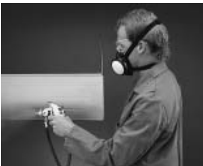
The versatile JGA-HVLP gun delivers a high quality finish with less overspray than conventional guns.
